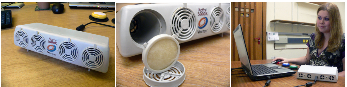
Figure 3.12: The olfactory device used in the experiment. This figure shows how the fabric disks were inserted into the device and how the device itself was positioned close to the user to minimise delivery time.
