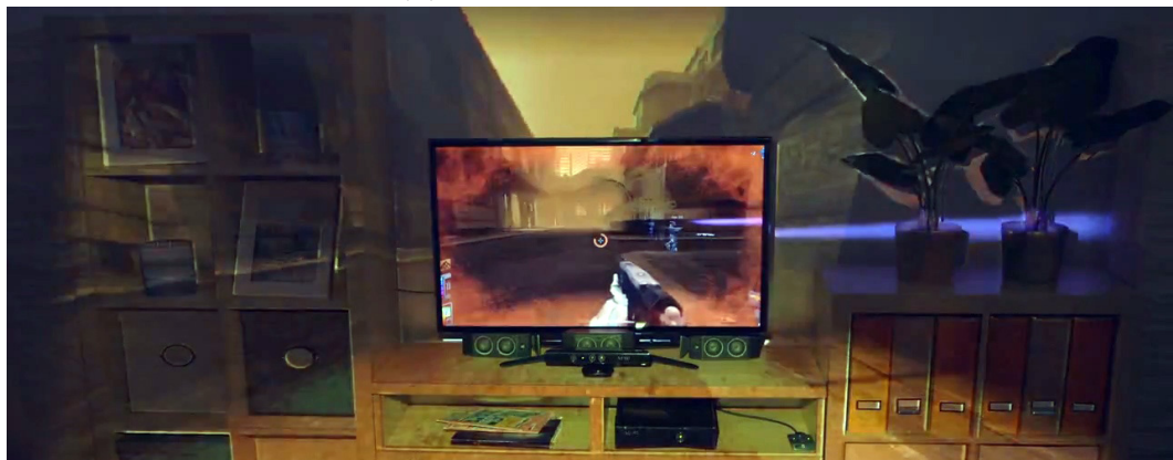
(b) The Microsoft Illumiroom. Note that the projection is distorted to ‘flatten’ furniture from the perspective of the user.
