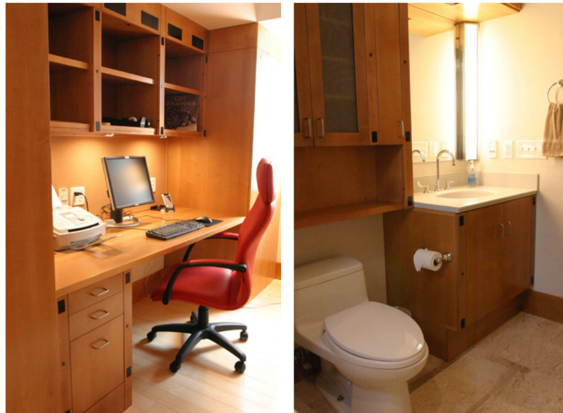
Figure 2.6: Photographs of the MIT PlaceLab from Intille et al. [102, p. 1942]. Each of the black squares shown in the pictures covers sensor circuitry. While the sensors themselves are not intrusive, the installation process would be disruptive.
